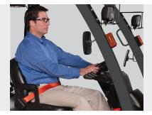
High Visibility Seatbelt Bright orange seatbelt provides instant visual confirmation that operators are using this safety equipment.
