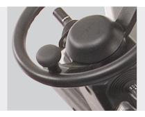
Steering Wheel Spinner Knob Provides easier operator control and handling.
