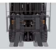
Sideshifting Fork Positioner Hydraulic fork adjustment prevents operator strain by eliminating the need to manually move forks for different pallet types for increased productivity.
