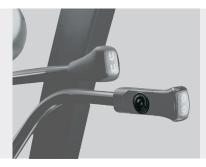
Auto-Tilt Leveling System Press the button on the hydraulic control lever to tilt the forks forward to a horizontal position. Used for easier load placement and retrieval operations.
