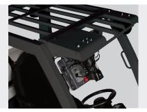
Extended Overhead Guard Extension provides protection to mounted components, including onboard computer and headlight (shown).
